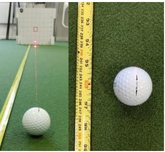
The ball should then be positioned in line with the laser. This should also be aligned with the centre of the ghost hole and the slot in the middle of the backboard. This should be 244 cm (8 feet) back from the centre of the ghost hole.
